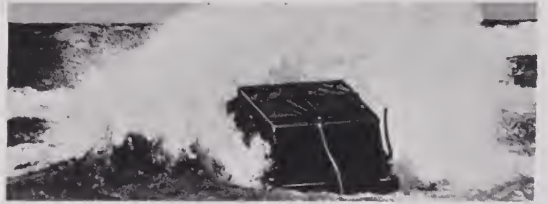
FIGURE 40. M-29C amphibious Weasel negotiating storm on Lake Michigan.
